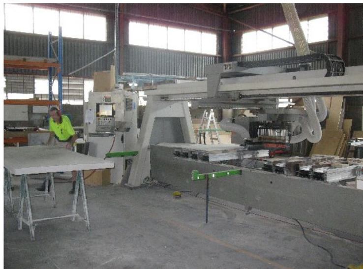
**CNC machine especially modified for fabrication of fibre cement products**
